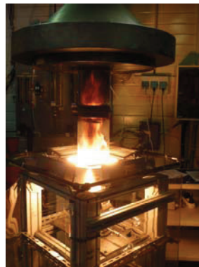
Figure 2a: Fire calorimetry testing of 2,5 DMF as a potential bio-sourced fuel component making use of the FPA (ISO 12136:2011)
