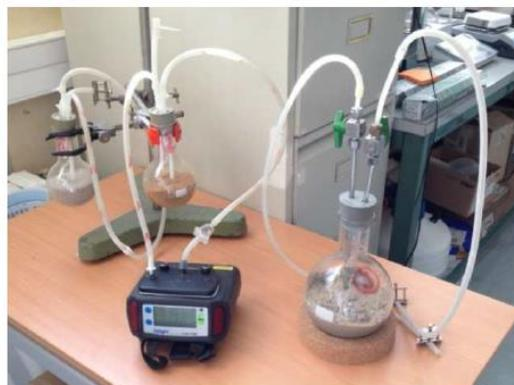
**Fig. 10** Experiments conducted in batches (Degrelle, 2012)
