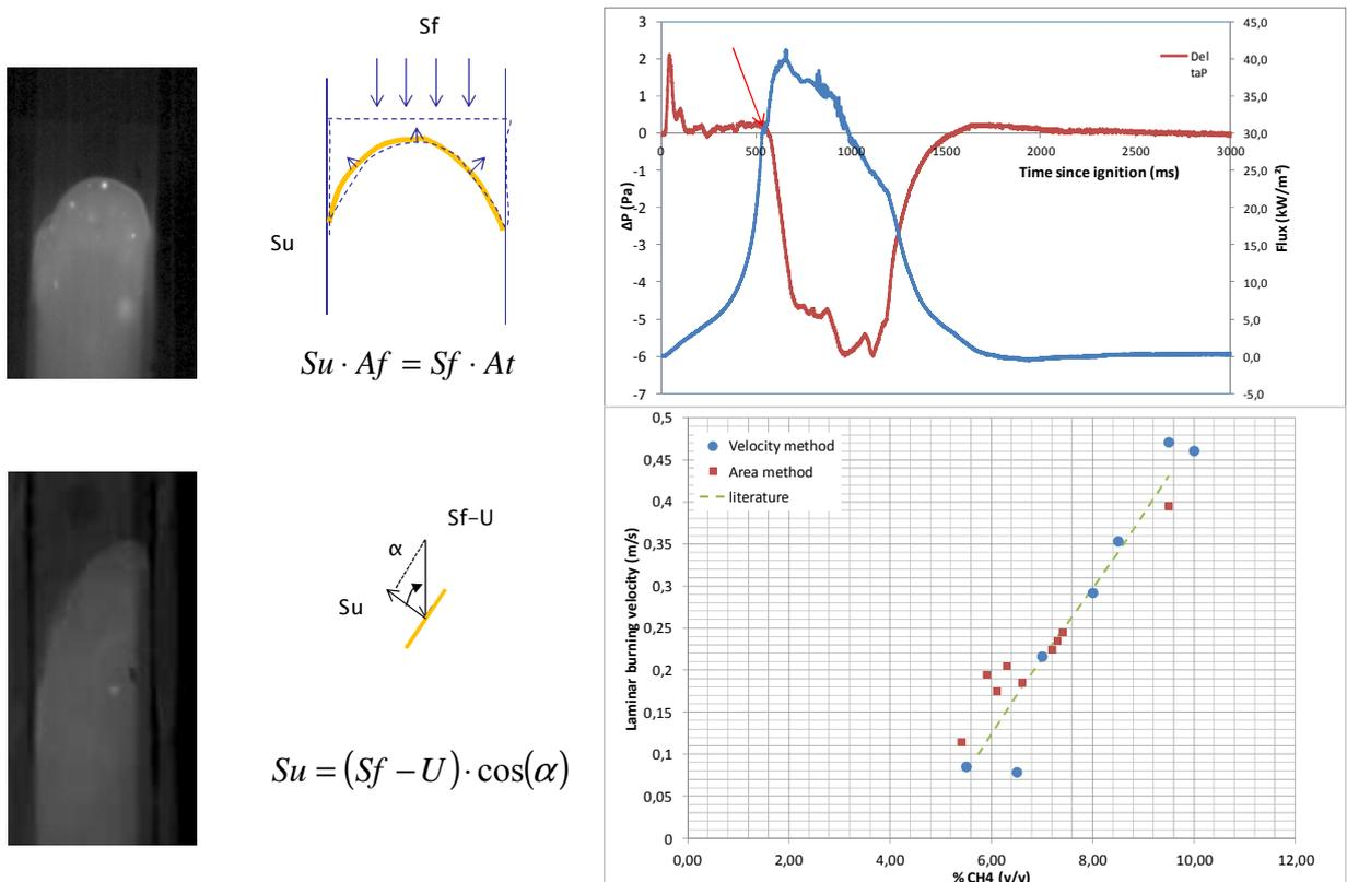
Figure 2 : laminar burning velocity methods
