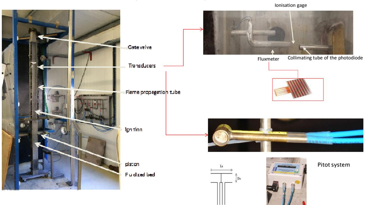
Figure 1. Experimental setup
