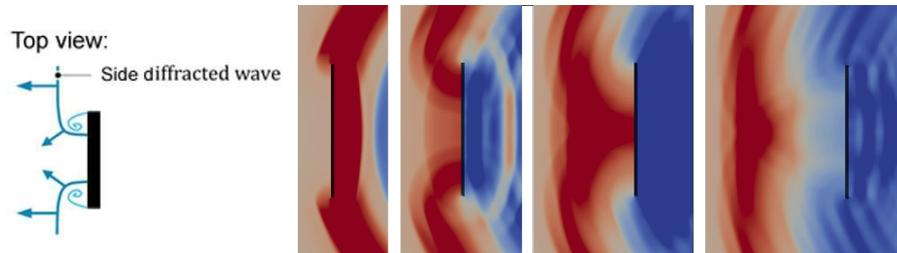
Figure 9: Left: Schematic representation of diffracted wave around an obstacle [7]. Right: Overpressure calculated with OPENFOAM between 50 and 65 ms (overpressure scale from -30 mbar (blue) to 30 mbar (red))
