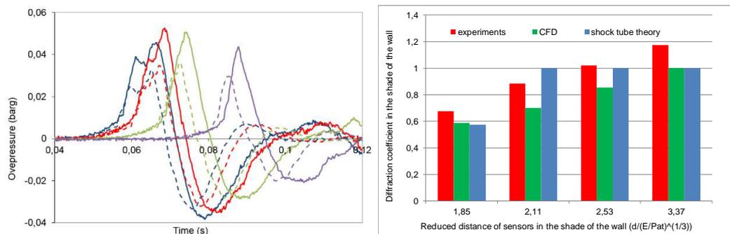
Figure 8: Left: experimental (line) and numerical (dash line) pressure signals 1 m (blue), 2.5 m (red), 5 m (green) and 10 m (purple) behind the wall. Right: overpressure measured and reduction coefficients behind the wall
