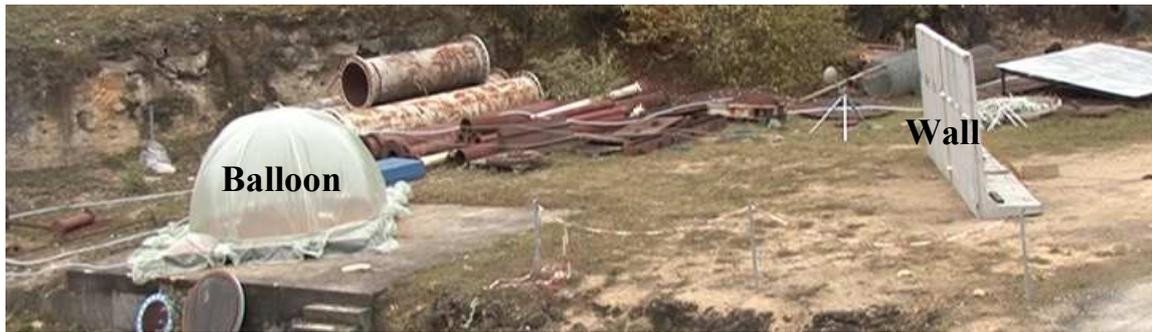
Figure 1: test platform with hemispherical balloon and protective wall of 6m length, 10 m between both
