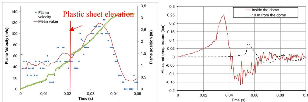
Figure 4: Left: flame trajectory (green dots) and velocity (blue dots and red line) on the vertical axis extracted from the film. Right: Overpressure measured by sensors inside the dome and 10m from the dome
