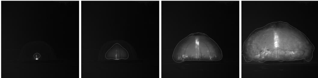
Figure 3: Processed images of the deflagration of the flammable mixture (10 ms between frames).
