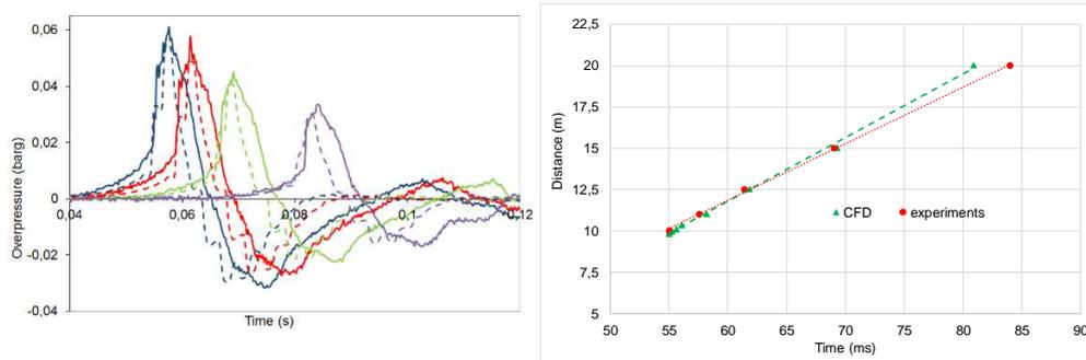
Figure 5: Left : Measured (lines) and CFD predicted (dots) overpressure between 11 and 20 m. Right: x-t diagrams of wave propagation
