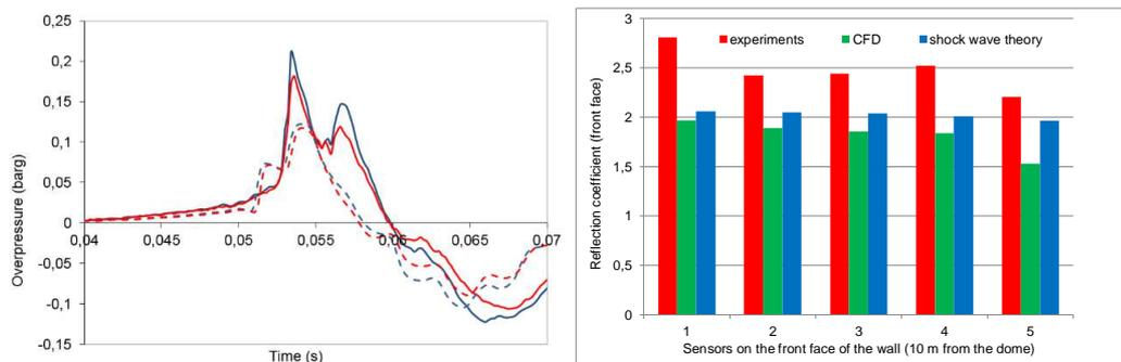
Figure 6: Left: Experimental (line) and calculated (dash line) pressure signals on sensors 1 (blue) and 2 (red) on the front face of wall. Right: Reflection coefficients on each wall sensor
