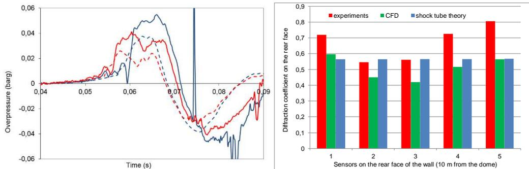
Figure 7: Left: experimental (line) and numerical (dash line) pressure signals on sensor 1 (blue) and 2 (red) on the rear face of wall. Right: overpressure measured and diffraction coefficients on the rear face of wall
