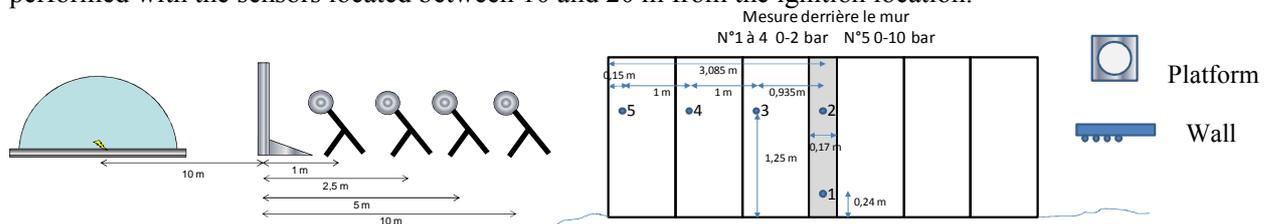
Figure 2: Location of pressure sensors in the shade and on the rear face of protective wall (the wall was reversed for incident directly impacting pressure wave measurements)
