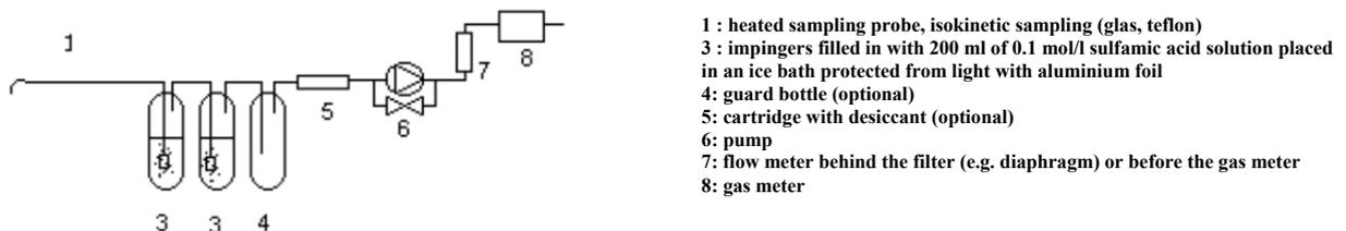
Figure 1: Sampling system used to collect atmospheric emissions
