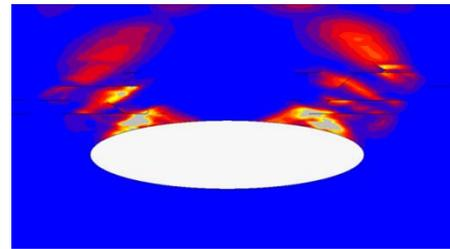
Figure 13: Effective plastic strain distribution with crack propagation.
