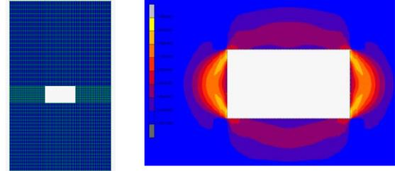
Figure 4: 2D finite elements mesh (left) and effective plastic strain (right) (L=30 m).
