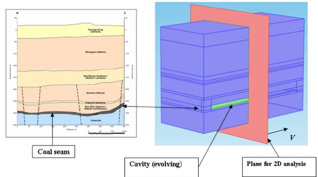
Figure 2: Stratigraphy and location of coal seam (on the left) and 3D numerical model (on the right). A 2D plane passing through the middle of exploitation used in plane strain numerical analyses.  $V$  stand for the burning front velocity.
