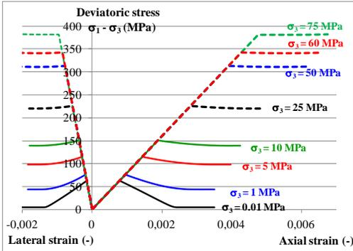
Figure 2: Numerical results of triaxial compression tests.
