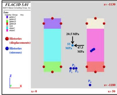
Figure 4: Geometrical model with position of history points.
