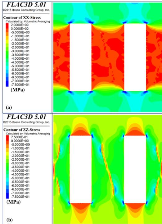
Figure 6: Horizontal (top) and vertical (down) stresses: model #1.
