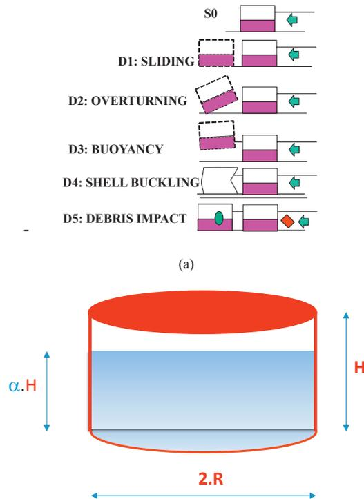
(b)- Tanks: 5 sizes {T<sub>1</sub>: H=8m, R=5.57m}; { T<sub>2</sub>: H=10m, R=14m}; { T<sub>3</sub>: H=19m, R=10m}; { T<sub>4</sub>: H=30m, R=20m}; { T<sub>5</sub>: H=30m, R=40m}
