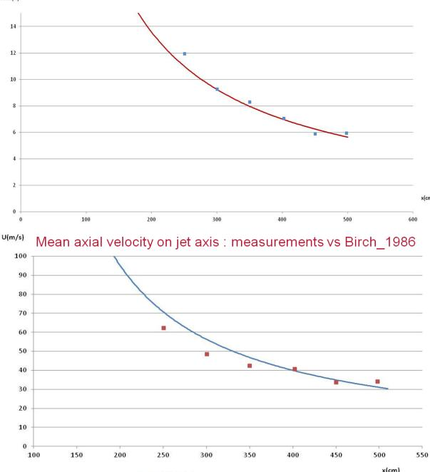
Figure 5: Axial decays of methane concentration and mean velocity axial for free jets tests carried out by INERIS and GDF SUEZ in 2011, compared to Birch correlations: (Birch, 1984); (Birch, 1987)
