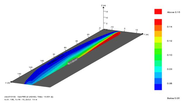
Figure 22: 3D cut plane of the jet release covering the congested area (volume concentration)
