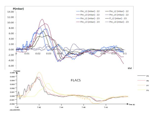
Figure 11: pressure signal over time for different sensors positions, measured in the free gas jet ignition test (top) and calculated by FLACS (bottom)
