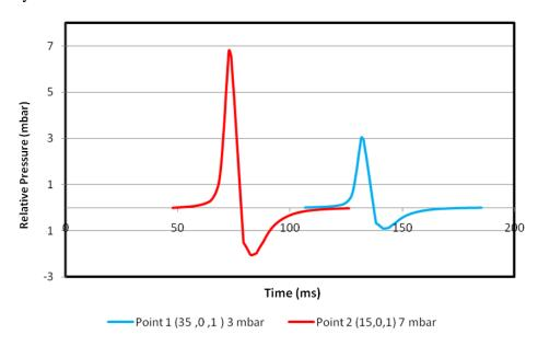
Figure 9: overpressure signals for 1 ignition test of a free methane jet
