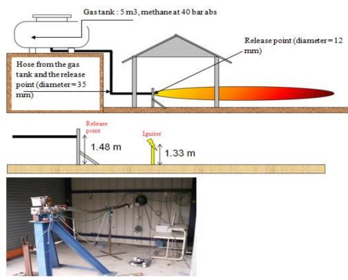
Figure 1: test bench used by INERIS and GDF SUEZ for free methane jets
