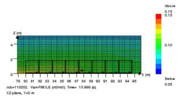
Figure 23: 2D cut plane of the gas concentration along the jet axis
