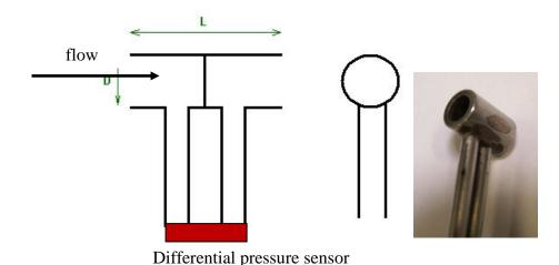
Figure 3: velocity probe: Bidirectional Pitot probe
