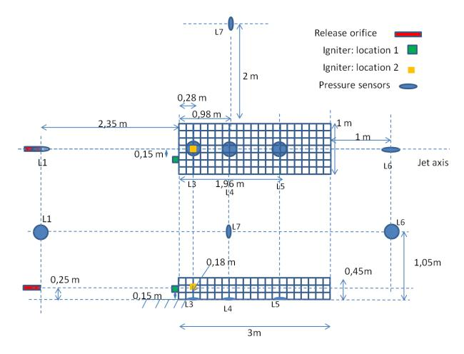
Figure 15: locations of the release orifice, pipes, igniter and pressure sensors used by INERIS and GDF SUEZ for methane jets within a 3D array of 20 mm diameter tubes
