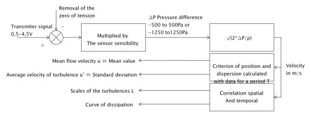
Figure 4: assessment of mean velocity, rms velocity and integral scale of turbulence from the signals of the differential pressure sensor mounted in the bidirectional Pitot probes
