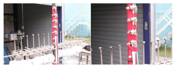
Figure 2: measurement devices: 11 oxygen sensors and 14 velocity probes (probes developed by INERIS based on McCaffrey probes)
