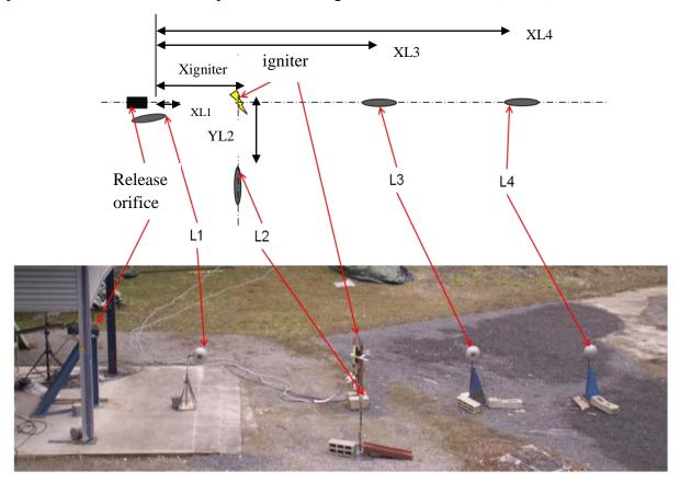
Figure 6: set-up of pressure sensors
