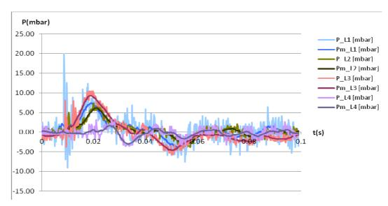
Figure 7: overpressure signals for 1 test of free jet
