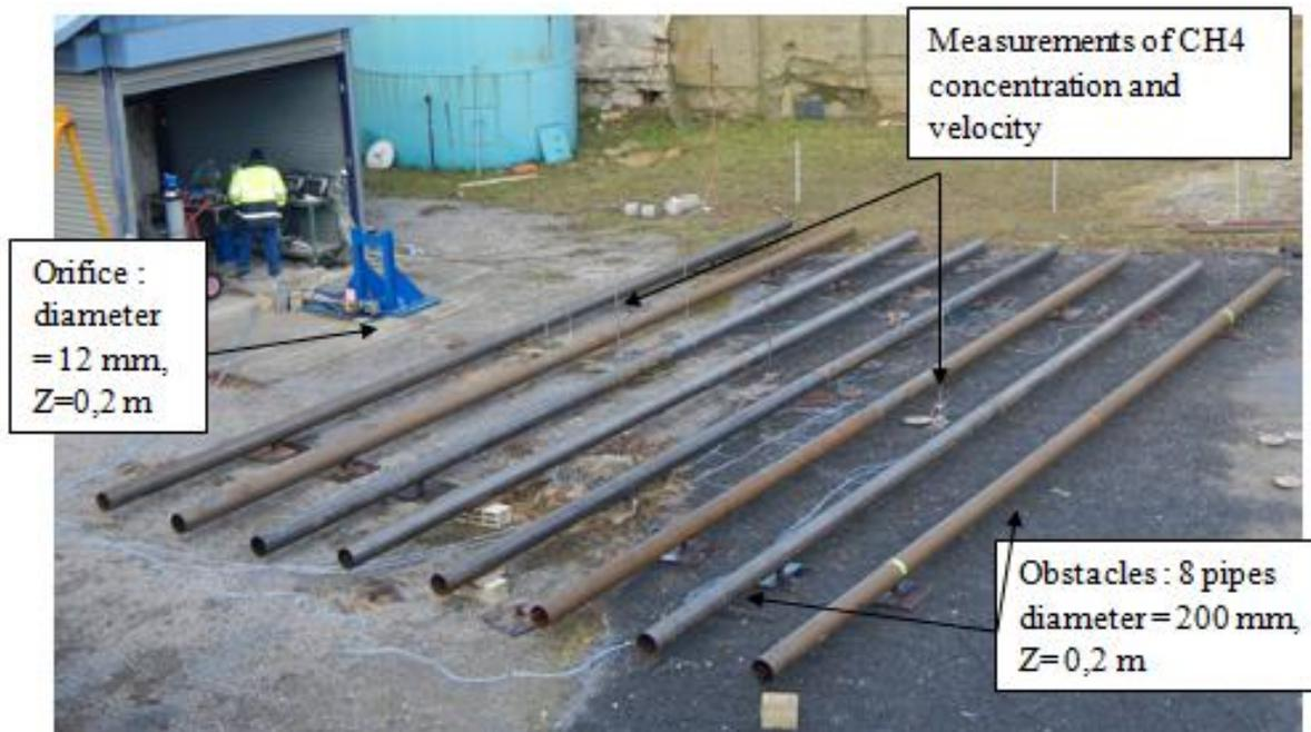
Figure 12 : test bench used by INERIS and GDF SUEZ for free methane jets
