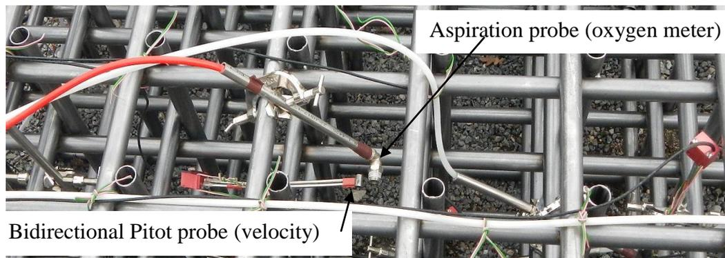
Figure 17 : aspiration probes and bidirectional Pitot probes used for the dispersion tests with the medium congestion module
