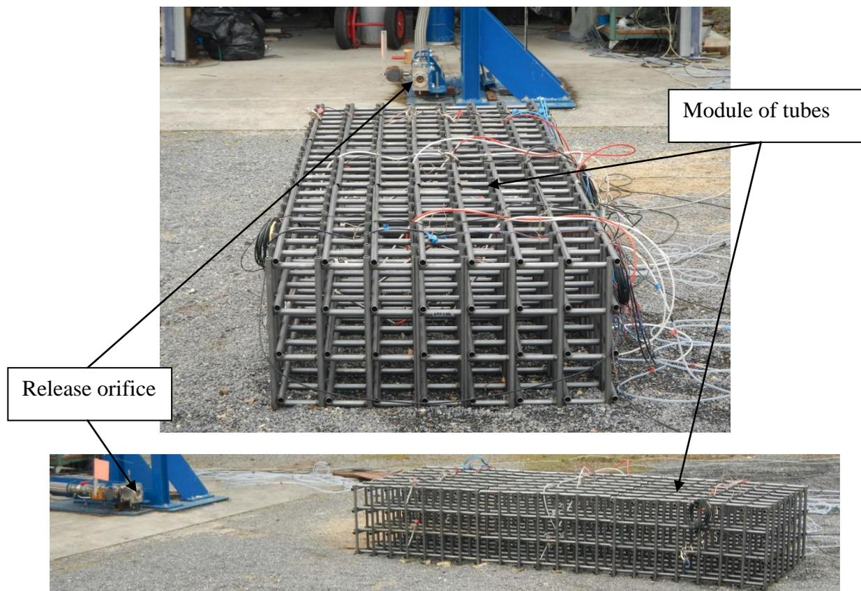
Figure 14 : 3D array of 20 mm diameter tubes used by GDF SUEZ and INERIS
