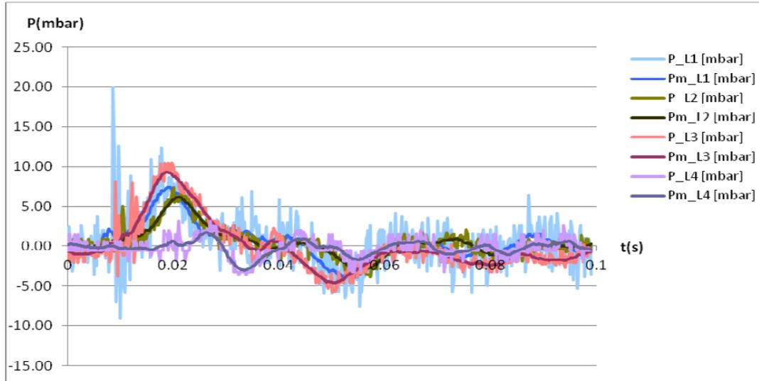
Figure 7 : overpressure signals for 1 test of free jet
