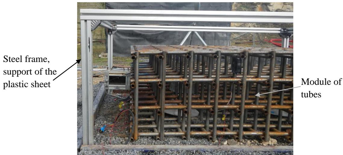
Figure 16 : steel frame which supports the plastic sheet, covering the module of tubes
