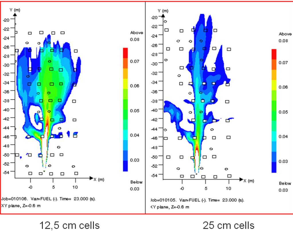
Figure 20 : dispersion calculation: comparisons of mean concentration fields for different meshes
