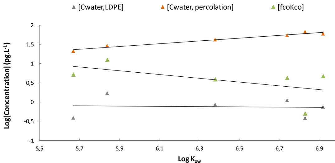
Figure 6: Concentrations of PCBs in pore water obtained by passive sampler (C<sub>water</sub> LDPE), percolation (C<sub>water</sub>, percolation) and by calculation with K<sub>d</sub> (fcoKco) for sediment of Marseille
