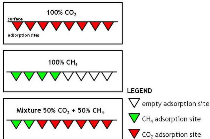
Fig. 5. Empirical model proposed by INERIS for the adsorption of CO<sub>2</sub> + CH<sub>4</sub> gas mixtures. Example with mixture “50%”.
