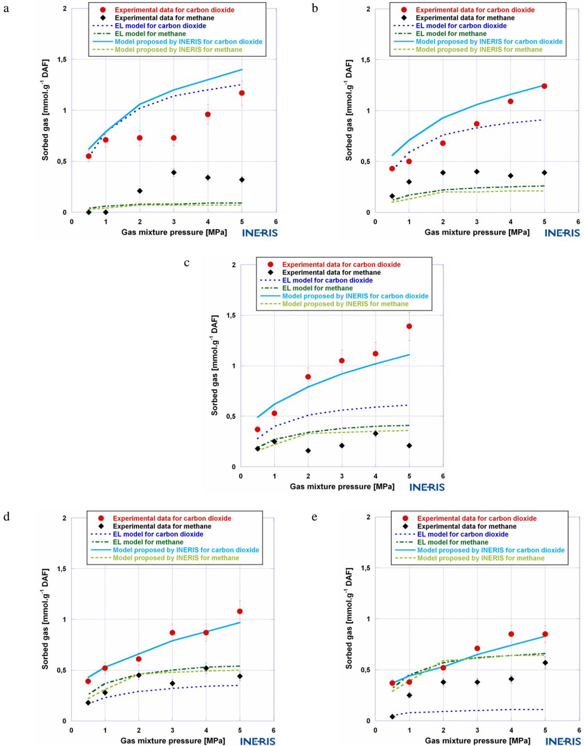
Fig. 6. Experimental results and theoretical isotherms for adsorption experiments of gas mixtures: (a) 90% CO<sub>2</sub> + 10% CH<sub>4</sub>; (b) 70% CO<sub>2</sub> + 30% CH<sub>4</sub>; (c) 50% CO<sub>2</sub> + 50% CH<sub>4</sub>; (d) 30% CO<sub>2</sub> + 70% CH<sub>4</sub>; (e) 10% CO<sub>2</sub> + 90% CH<sub>4</sub>.
