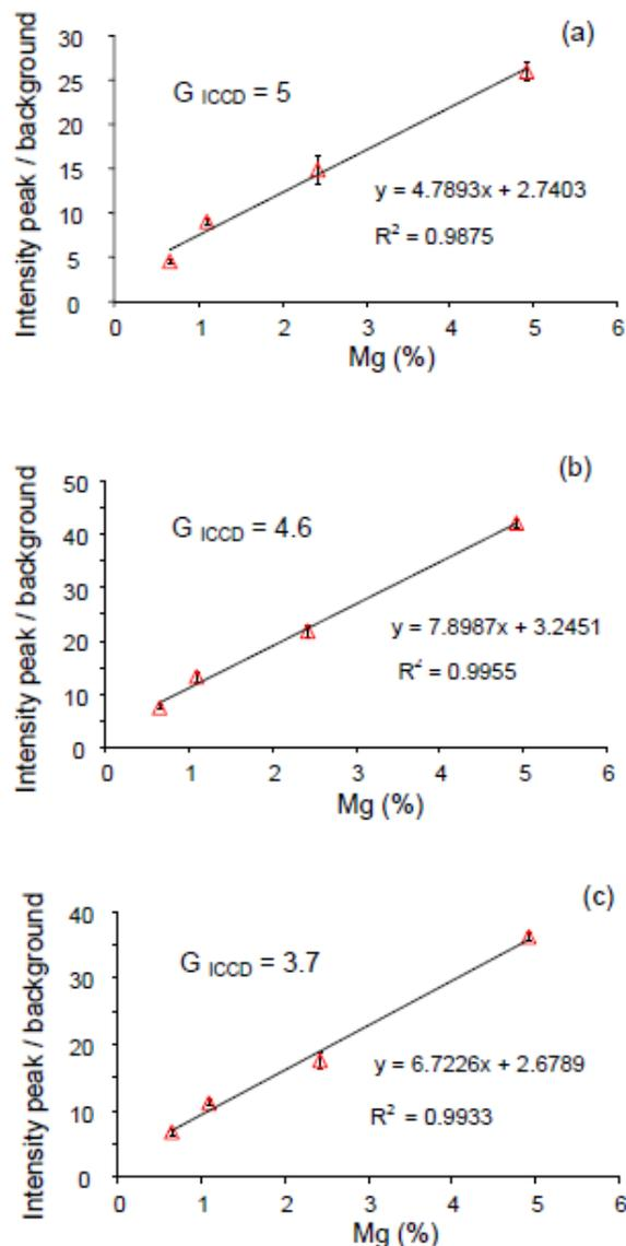
**Figure 13.** Mg calibration curve ( $\lambda=518.36$  nm) for Al matrix samples with Mg-concentrations (4.9%, 2.4%, 1.1%, 0.65%) under 1 ps microablation (100  $\mu$ J, 30 shots per crater): (a) – single pulse in air; (b) – double pulses in air; (c) – double pulses with Ar-jet.  $G_{ICCD}$  - the applied ICCD camera gain.
