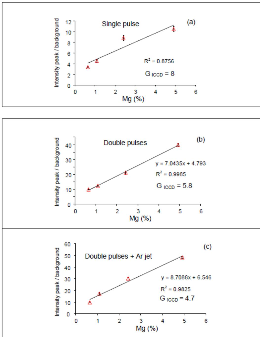
**Figure 9.** Mg calibration curves ( $\lambda=518.36$  nm) for Al matrix samples with different Mg mass content (4.9%, 2.4%, 1.1%, 0.65%) under 50 fs microablation (40  $\mu$ J, 30 shots per crater): (a) – single pulse in air; (b) – double pulses in air, (c) – double pulses with Ar-jet.  $G_{ICCD}$  - the applied ICCD camera gain.
