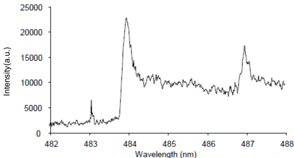
**Figure 11.** AIO spectrum for Al sample under 50 fs microablation in air (40  $\mu$ J, single pulse).
