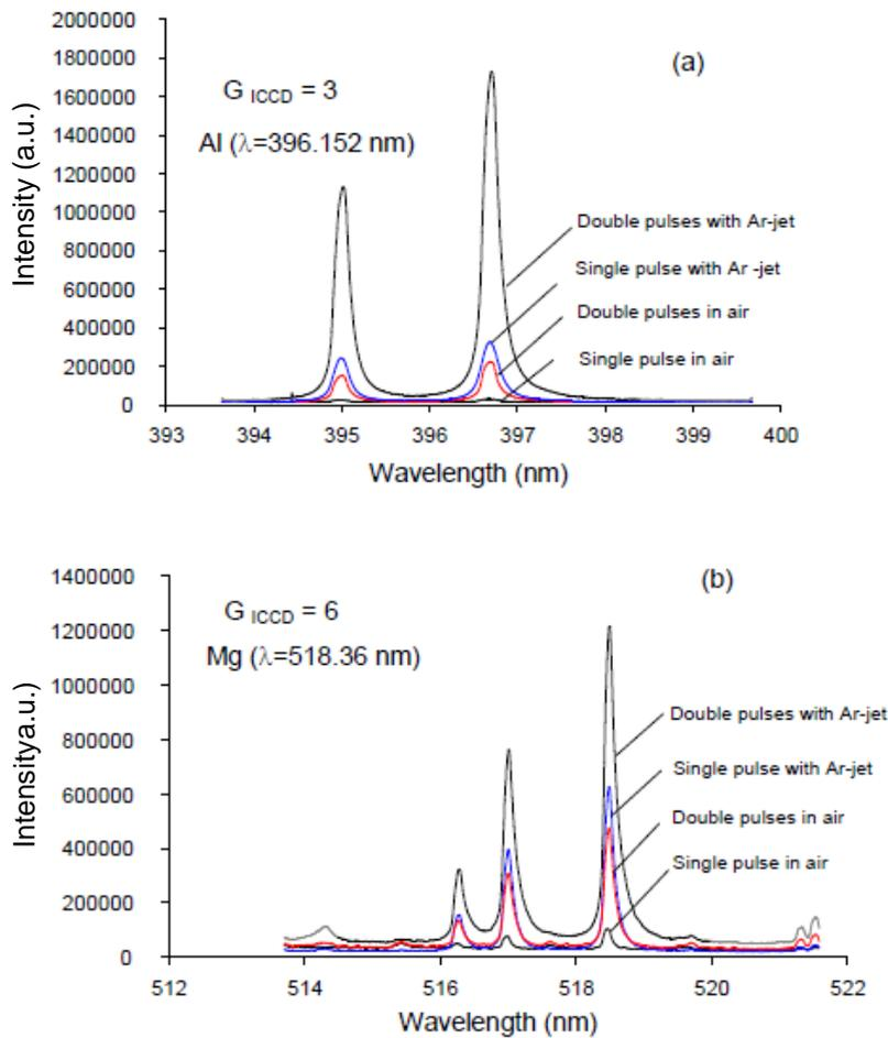
**Figure 8.** (a) - Al ( $\lambda=396.152$  nm) and (b) - Mg ( $\lambda= 518.36$  nm) spectral line intensity for the polished Al matrix sample (with Mg of 1.5 % mass content) under 50 fs microablation (40  $\mu$ J, single and double pulses, in air and with Ar-jet).  $G_{ICCD}$  - the applied ICCD camera gain.
