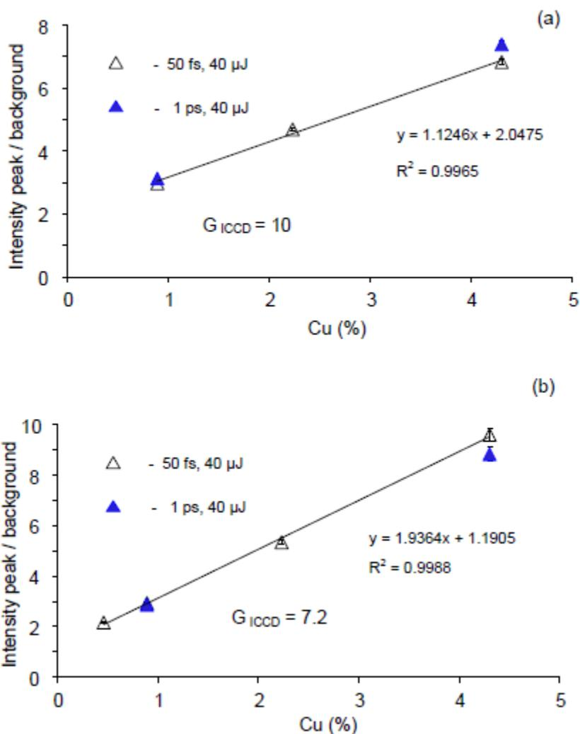
**Figure 10.** Cu calibration curves ( $\lambda = 521.82$  nm) for Al matrix samples with different Cu mass content (4.3%, 2.2%, 0.9% and 0.46%) under 50 fs and 1 ps microablation (40  $\mu$ J, 30 shots per crater): (a) – double pulses in air; (b) – double pulses with Ar-jet.  $\Delta$  - 50 fs;  $\blacktriangle$  - 1 ps.  $G_{ICCD}$  - the applied ICCD camera gain.
