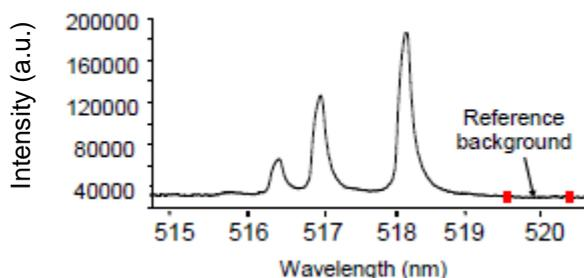
**Figure 14.** Mg spectrum (accumulated after 30 shots) for Al matrix sample with a low Mg concentration (0.65%) under 1 ps microablation (100  $\mu$ J, double pulses, with Ar-jet). The standard deviation of the background intensity was calculated within the spectral zone indicated by two dots. The ICCD camera gain  $G_{\text{ICCD}} = 3.7$ .
