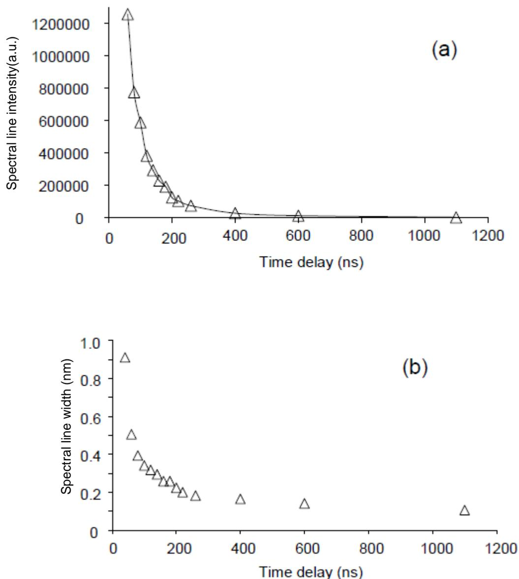
**Figure 3.** (a) – temporal evolution of Al spectral line intensity ( $\lambda = 396.15$  nm) in arbitrary units and (b) - spectral line width (FWHM) in nm versus the ICCD camera time delay for 50 fs microablation of the polished Al sample (40  $\mu$ J, single pulse, in air, ICCD camera gate width  $t_g = 20$  ns).
