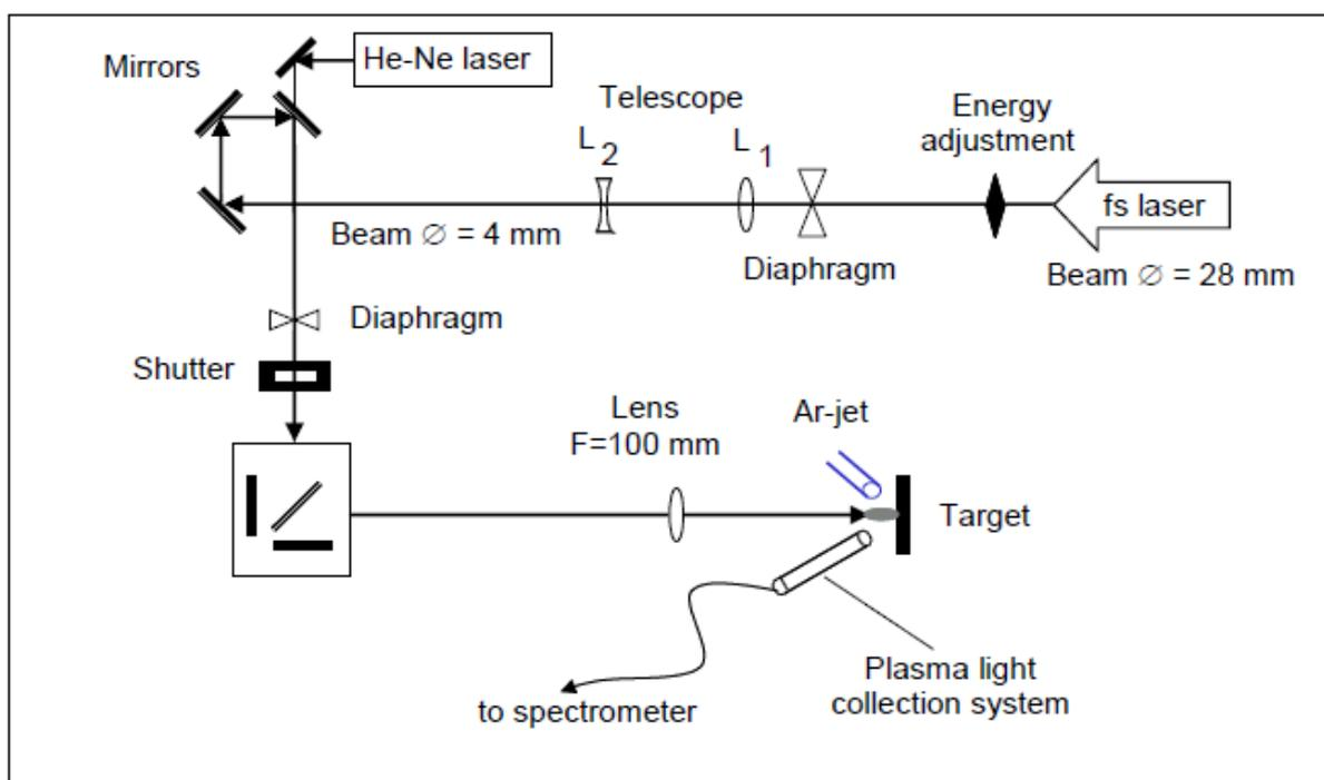
**Figure 1.** Diagram of the experimental setup for micro-LIBS measurements.
