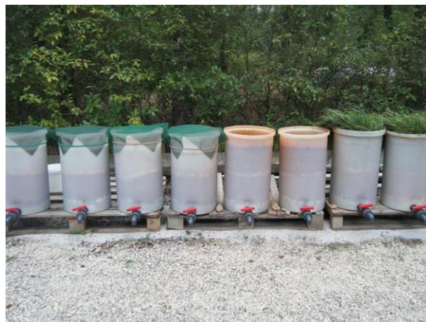
Figure 7: Lysimeters of spent MBR with different top layer
