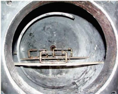
*Perforated ring of the 1 m<sup>3</sup> vessel*
