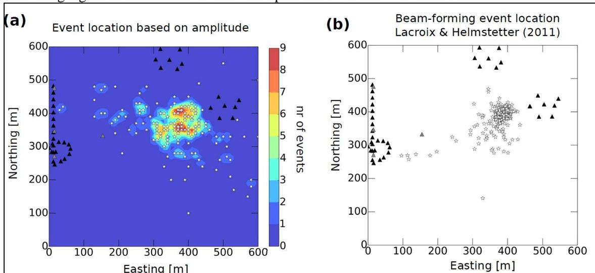
Figure 1: Example of event location results using an amplitude based (a) (Kinscher et al 2015) and a beam-forming based (b) (Lacroix & Helmstetter 2011) approach for ~ 250 events detected on the 20/10/2013. Black triangles refer to seismic stations of the permanent OMIV network, while gray triangles mark station positions of the temporal INERIS network.
