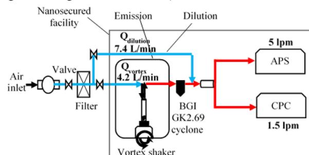
**Fig. 1.** Schematic of the vortex shaker experimental setup.
