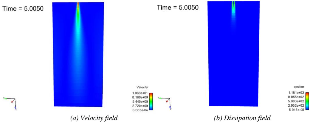
Figure 2. Qualitative result of fluid phase. (a) Velocity field. (b) Dissipation field. Time simulation is 5 s.
