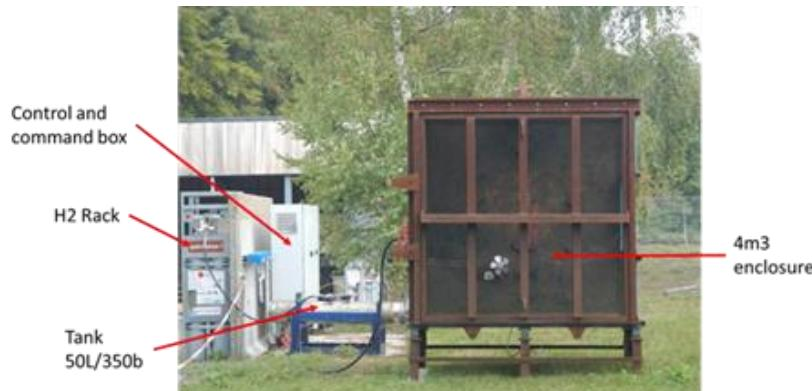
Figure 2. Illustration of the experimental set-up
