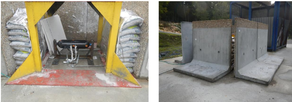
Figure 6. Outdoor experimental setup for hydrogen use (confinement not yet in place in left picture)
