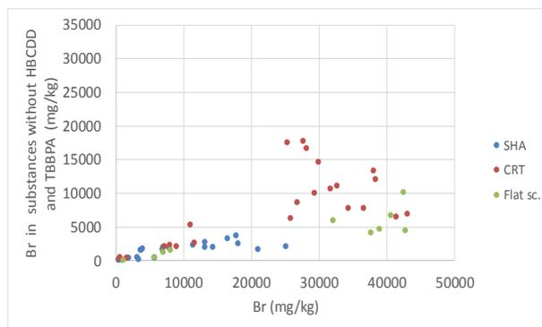
Figure 6: Bromine in measured substances (excepted HBCDD and TBBPA) as a function of total bromine in WEEE (2015) (n=56 with triplicates)
