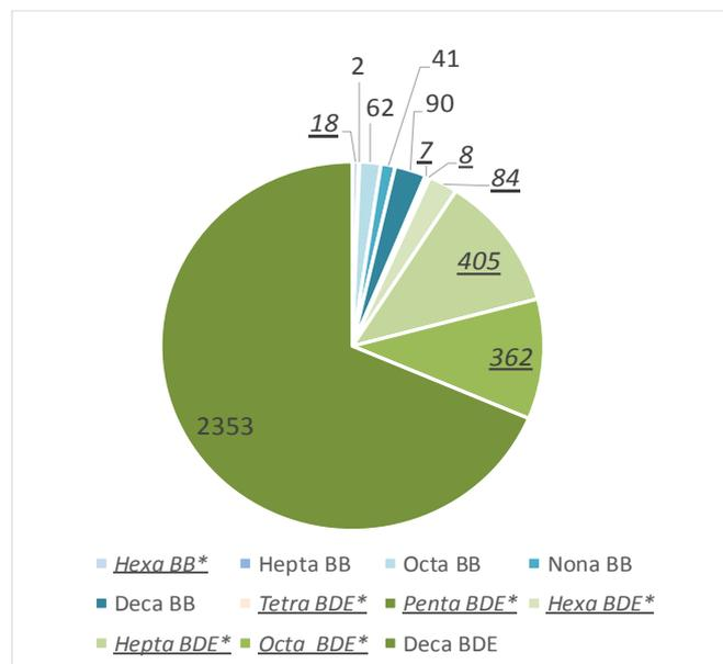
Figure 2: Concentration of brominated flame retardants in WEEE 2014 (mg/kg, n = 33, values > LOQ, PBBs and PBDEs < LOQ not represented, HBCDD and TBBPA not measured; \* classified substances are underlined)
