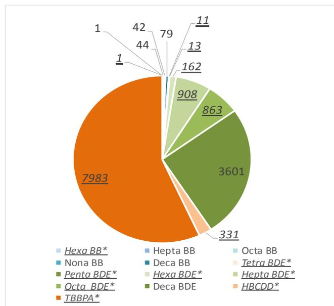
Figure 3: Concentration of brominated flame retardants in WEEE 2015 (mg/kg, n = 32, values > LOQ, PBBs and PBDEs < LOQ not represented; \* classified substances are underlined)
