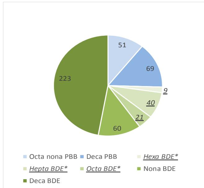
Figure 1: Concentration of brominated flame retardants in EEE 2009-2013 (mg/kg, 32 parts of 22 equipment, PBBs and PBDEs < LOQ not represented, HBCDD and TBBPA not measured; \*classified substances are underlined)
