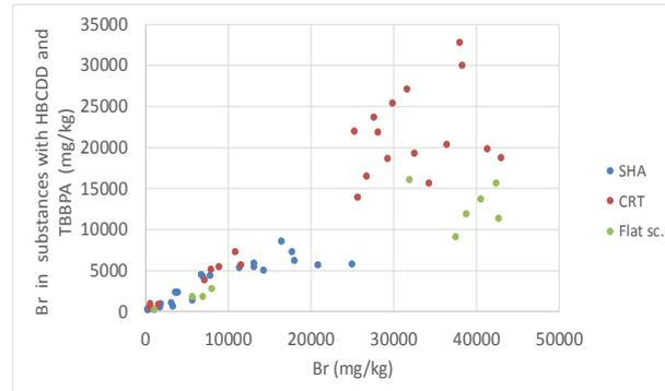
Figure 7: Bromine in measured substances (including HBCDD and TBBPA) as a function of total bromine in WEEE (2015) (n=56 with triplicates)
