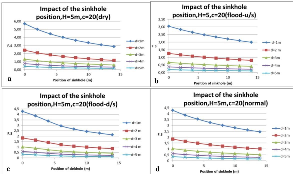
Figure 5. Relation between the position of cavity with respect to the dike and the safety factor. a- dry case (water level below of alluvial layer), b- flood case for the
