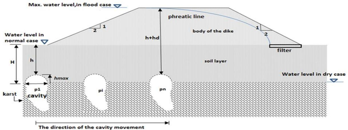
Figure 4. Different positions of sinkhole (horizontally from position  $p_1$  to position  $p_n = 14$  m)
