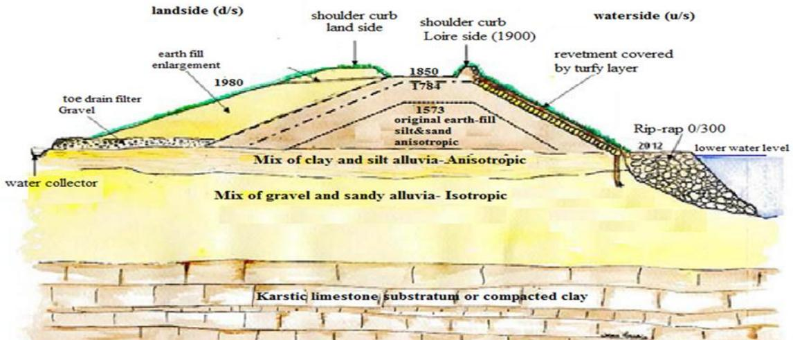
Figure 3. Typical cross section of a Loire levee nowadays (courtesy Jean Maurin) (International Levee Handbook, 2012)
