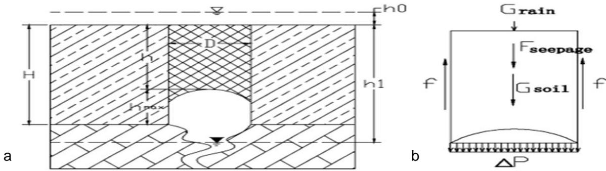
Figure 2. (a) Cross section of the karsts collapse column, (b) Mechanical analysis of the karsts collapse column (He Keqiang et al, 2004).
