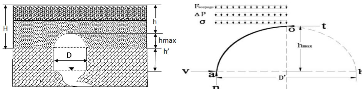
Figure 1. (a)Original karsts cave and equilibrium arc of the soil hole. Where  $h_{max}$  refers to the height of the pressure arch above the cave ceiling, which is the limit equilibrium height of a soil-hole arch; and  $H$  is the thickness of cover-layer soil (one layer or more) (He Keqiang et al, 2004). (b) Mechanical condition of the pressure arch (He Keqiang et al, 2004)
