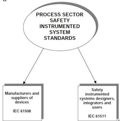
Figure 3: Scope of IEC 61508 / IEC 61511
