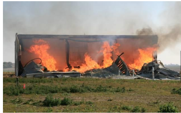
61 min after ignition : the structure of the cell submitted to fire has totally collapsed except for the fire-resistant concrete wall
