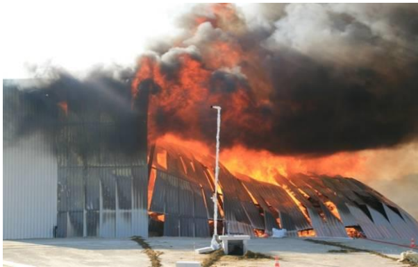
30 min after ignition : the structure collapses toward the inside
