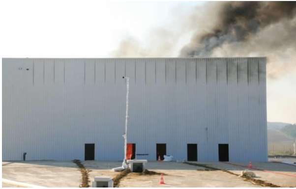
11 minutes after ignition : opening of the first smoke exhaust, opening of the second exhaust 1 min later
