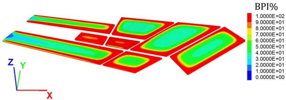
Fig. 7. Rockburst tendency at shaft station level (BPI criterion).
