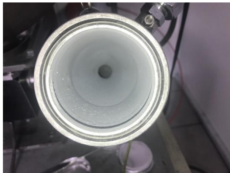
Figure 6: Injection reservoir covered with alumina after the pre-ignition of nano-aluminum
