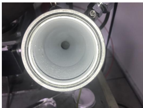
Figure 6: Injection reservoir covered with alumina after the pre-ignition of nano-aluminum
