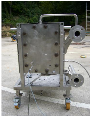
Picture 4. The protective casing was partially torn off.
