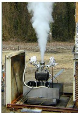
Picture 3. Picture of 10-liter test reactor.
