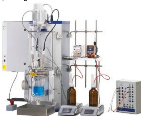
Picture 1. Picture of reaction calorimeter RC1.
