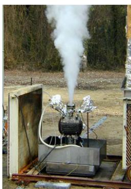
Picture 3. Picture of 10-liter test reactor.
