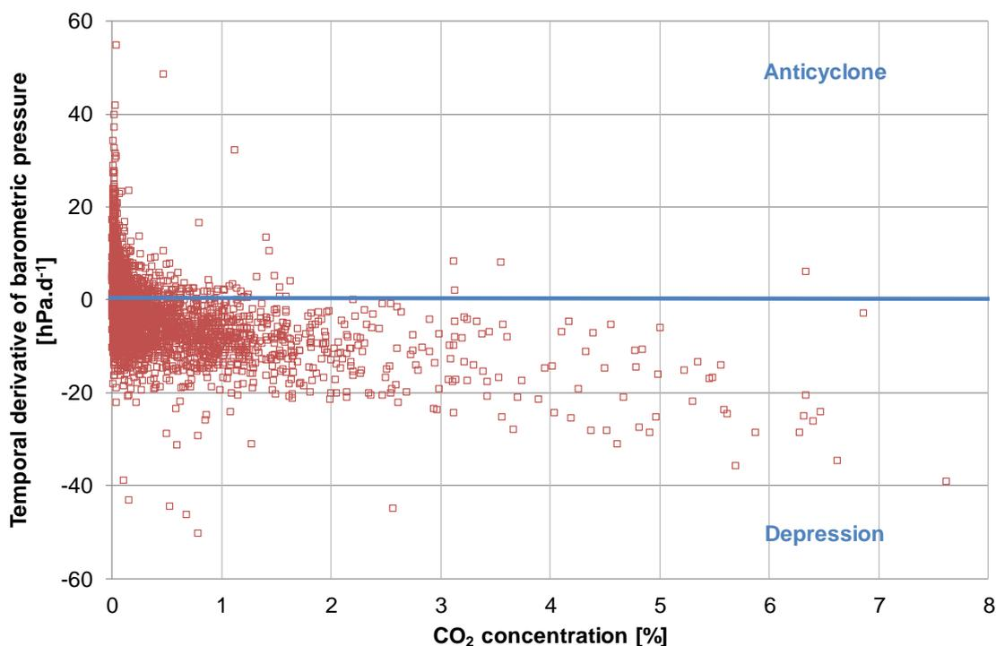
Figure 3. Temporal derivative of the barometric pressure versus the CO<sub>2</sub> concentration in a fracture at surface in the “Cité Belle Roche”.
