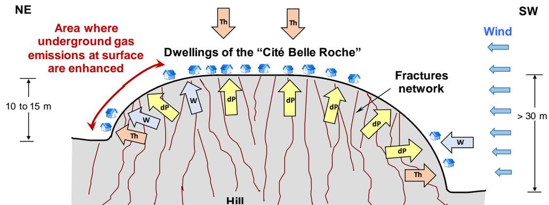
Figure 6. Schematic diagram of the combined action of a depression (dP; yellow arrows), thermal draught (Th; orange arrows) and prevailing wind (W; blue arrows) in the “Cité Belle Roche” during summer.
