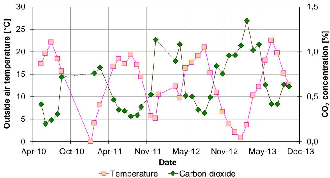
Figure 4. Influence of the natural thermal draught on CO<sub>2</sub> concentration in a fracture at surface in the “Cité Belle Roche”.
