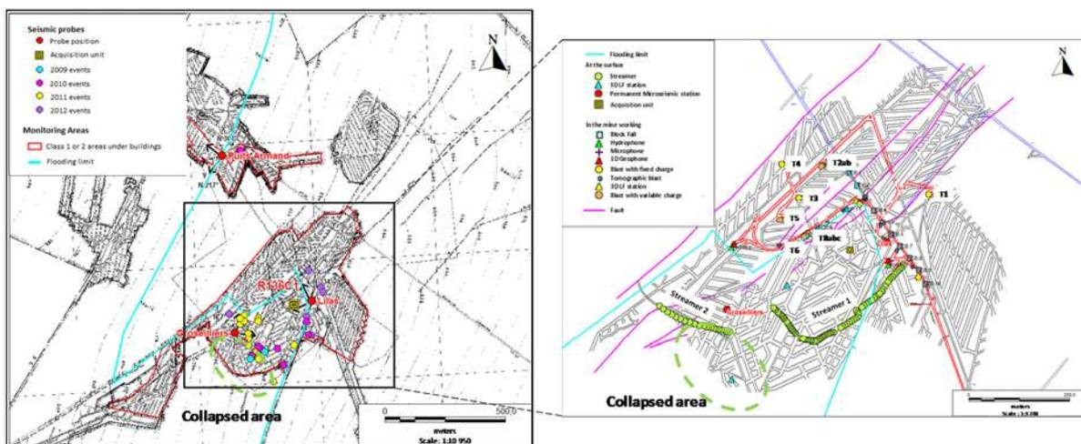
Figure 2 left map: mine workings of the iron ore grey layer of the site and location of the risk zone (red lines) and the permanent microseismic network (red points). Right map: Location of the different acquisition system and the blast superimposed to the grey layer mine workings (BRGM-DPSM)
