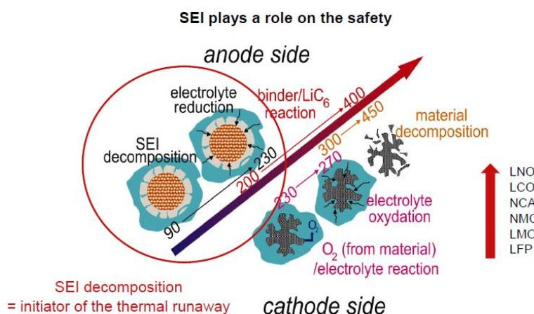
Fig. 1: underpinning phenomena in the process of thermal runaway of a li-ion cell according to chemistry (adapted from ref.[2])
