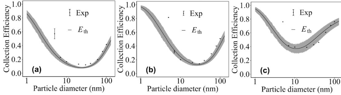
Fig. 6. Uncertainty analysis of 100 nm particle sampling efficiency in the conditions of (a) changing pore size; (b) changing flowrate; (c) changing particle density.
