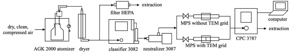
Fig. 2. Experimental set-up
