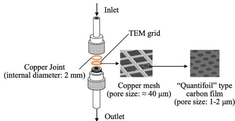
Fig. 1. Concept diagram of the TEM grid-equipped MPS
