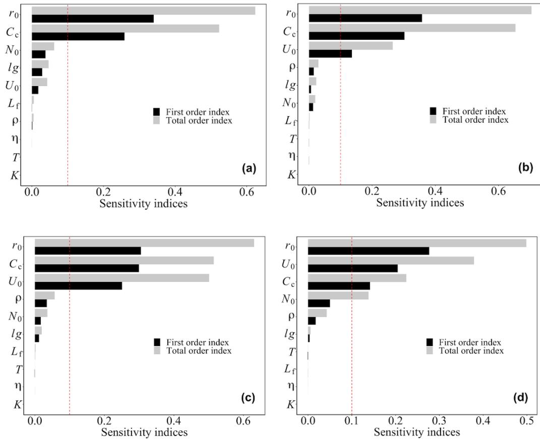
Fig. 5. Parameter sensitivity analysis of the NaCl particle sampling efficiency for sizes of (a) 10 nm; (b) 20 nm; (c) 50 nm; and (d) 100 nm.
