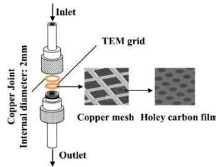
Fig. 10. Structure of MPS (Ogura et al., 2014)
