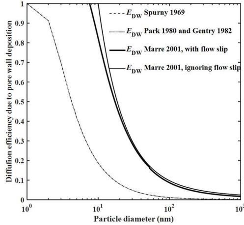
Fig. 3. Theoretical models of diffusion efficiency due to pore wall deposition (models of Spurny and Gentry overlap) ( $r_0 = 1 \mu\text{m}$ ,  $P = 0.1$ ,  $L_f = 9 \mu\text{m}$ ,  $U_0 = 2 \text{ m/s}$ ,  $\rho_p = 2000 \text{ kg/m}^3$ )
