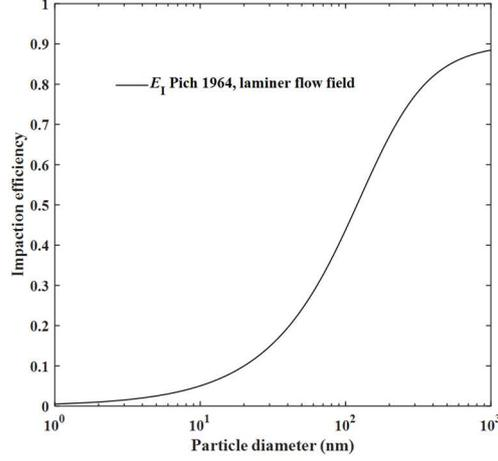
Fig. 6. Theoretical models of impaction efficiency ( $r_0 = 1 \mu\text{m}$ ,  $P = 0.1$ ,  $L_f = 9 \mu\text{m}$ ,  $U_0 = 2 \text{ m/s}$ ,  $\rho_p = 2000 \text{ kg/m}^3$ )
