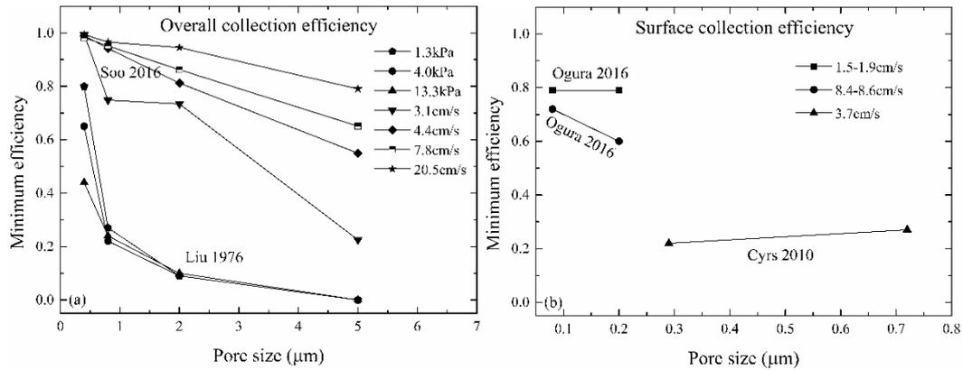
Fig. 7. Effect of pore size on collection efficiency
