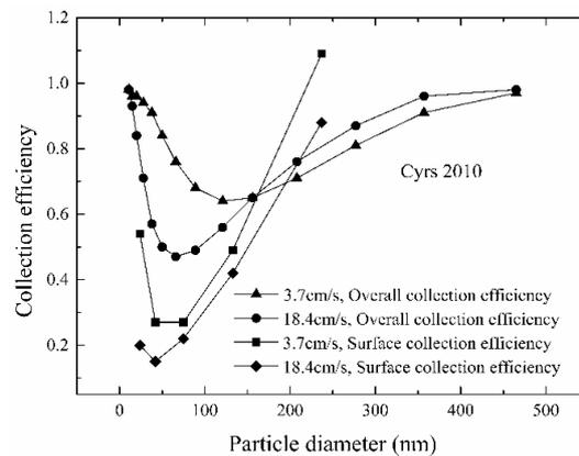
Fig. 8. Effect of face velocity on collection efficiency
