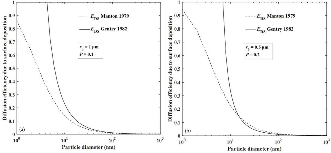
Fig. 4. Theoretical models of diffusion efficiency due to surface deposition ( $L_f = 9 \mu\text{m}$ ,  $U_0 = 2 \text{ m/s}$ ,  $\rho_p = 2000 \text{ kg/m}^3$ ; and (a)  $r_0 = 1 \mu\text{m}$ ,  $P = 0.1$ ; (b)  $r_0 = 0.5 \mu\text{m}$ ,  $P = 0.2$ )
