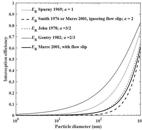
Fig. 5. Theoretical models of interception efficiency ( $r_0 = 1 \mu\text{m}$ ,  $P = 0.1$ ,  $L_f = 9 \mu\text{m}$ ,  $U_0 = 2 \text{ m/s}$ ,  $\rho_p = 2000 \text{ kg/m}^3$ )
