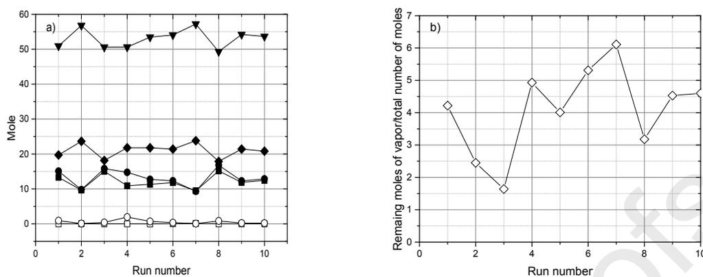
**Figure 8.** a) pyrolysis at 2500 K and 1 bar of methane (40%  $v/v$ ) in oxygen containing 100 moles of reactants (case with 6 components, 10000 composition vectors H<sub>2</sub>O, ▼; CO, ◆; H<sub>2</sub>, ●; CO<sub>2</sub>, ■; O<sub>2</sub>, ○; CH<sub>4</sub>, □); b) condensation at 1 bar – 250 K of an alcoholic solution containing 100 moles of mixture (case with 8 components; 10000 composition vectors) where  $N_R$  is remaining moles of vapor, ◇.
