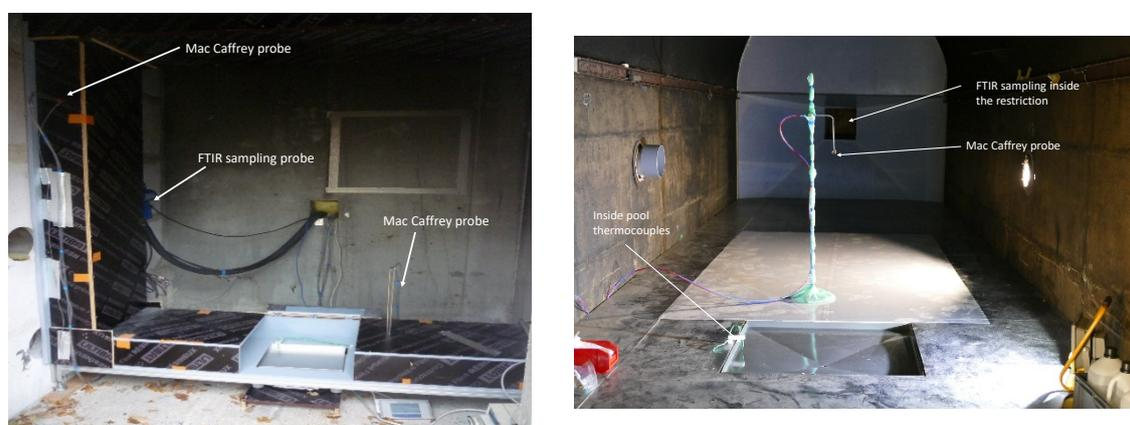
**Figure 2.** Picture of the pool photography and instrumentation for small (**left**) and medium (**right**) scales.
