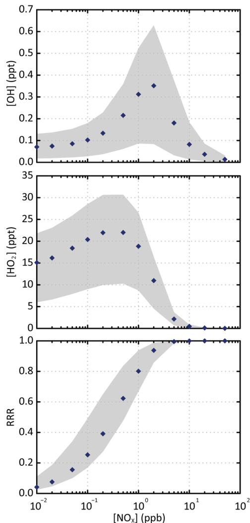
**Figure 1.** Simulated stationary state concentration of OH and HO<sub>2</sub> and corresponding reaction rate ratio (RRR) as a function of NO<sub>x</sub> concentrations for the various scenarios. The blue points are the simulated values for the scenario performed at a temperature of 298 K, a zenith angle of 50° and 40 ppb of ozone. The grey zone corresponds to the range of values simulated in all the scenarios.
