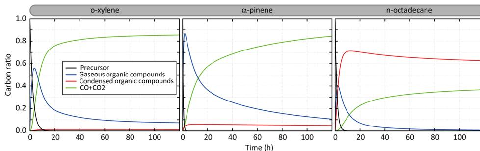
**Figure 2.** Temporal evolution of the simulated carbon distribution between the precursor, CO and CO<sub>2</sub>, and gaseous and condensed organic compounds. Simulated results are shown for o-xylene,  $\alpha$ -pinene and n-octadecane for the scenario performed at a temperature of 298 K, a zenith angle of 50°, a  $C_{\text{Oa}}$  of  $1 \mu\text{g m}^{-3}$ , 40 ppb of ozone and a RRR of 90 %.
