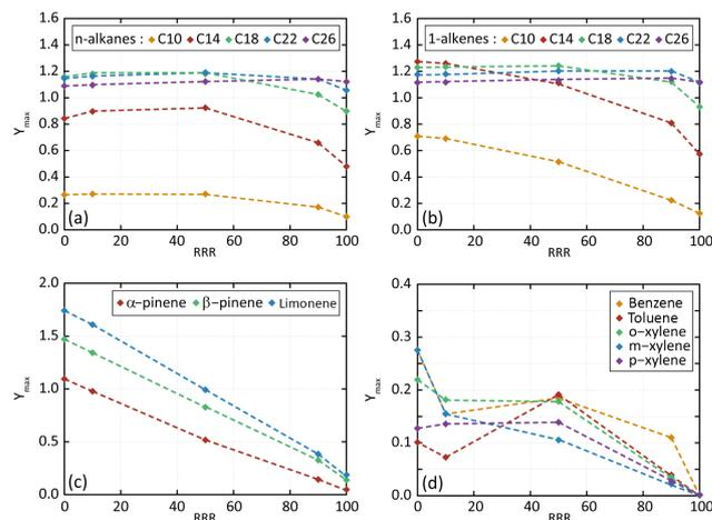
**Figure 4.** Dependence of  $Y_{\max}$  on RRR (here in percent) for n-alkanes (a), 1-alkene (b), terpenes (c) and aromatic species (d) for the scenarios performed at a temperature of 298 K, a zenith angle of  $50^\circ$ , a  $C_{\text{Oa}}$  of  $1 \mu\text{g}\cdot\text{m}^{-3}$  and 40 ppb of ozone. Points are connected with dashed lines to help in seeing trends of  $Y_{\max}$  with RRR.
