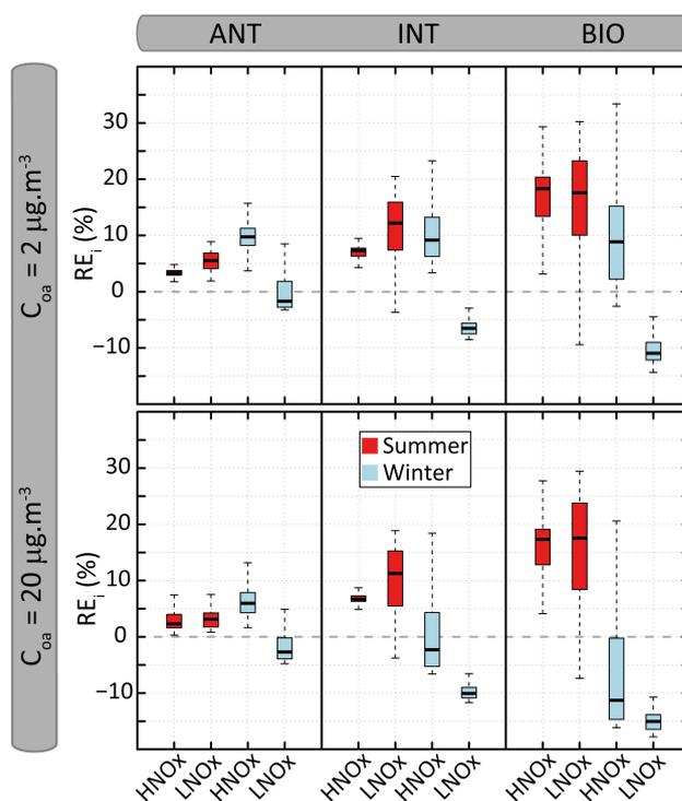
**Figure 9.** Distribution of the relative errors ( $RE_i$ ) on organic aerosol mass concentration calculated between VBS-GECKO and GECKO-A for the 24 evaluation scenarios. The bottom and top of the boxes are the first and third quartiles; the bands inside the boxes represent the medians. The ends of the whiskers represent the lowest and the highest  $RE_i$  values. There are 361 time steps for each evaluation scenario.
