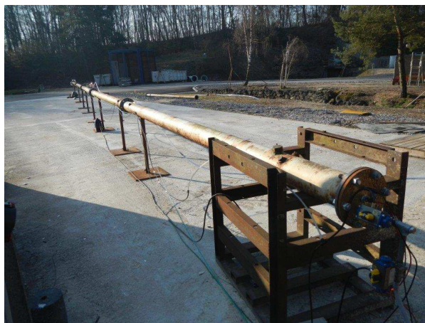
Figure 1: View of the experimental set-up. Top: PMMA pipe, with a 250-mm inner diameter. Bottom: metal pipe, with a 150-mm inner diameter.
