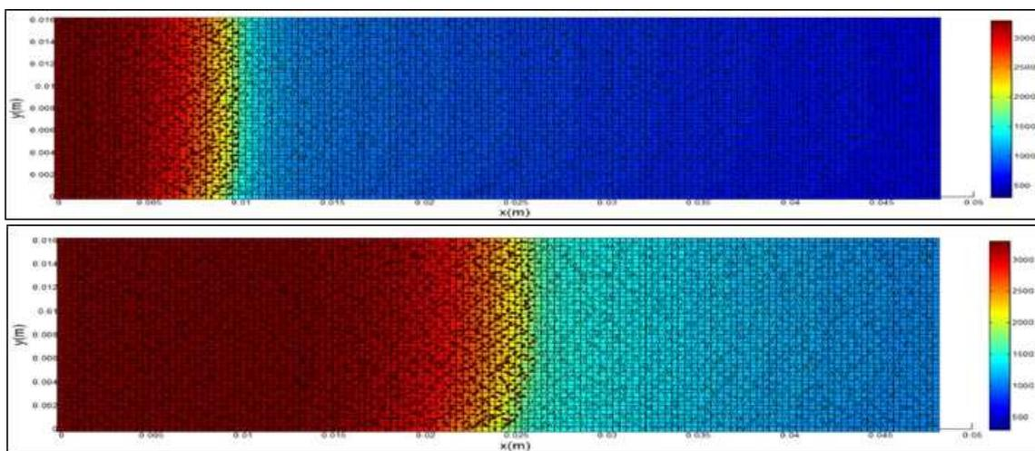
**Fig. 11:** Zoom on temperature field, Al dust-air flame,  $C_d = 500 \text{ g/m}^3$
