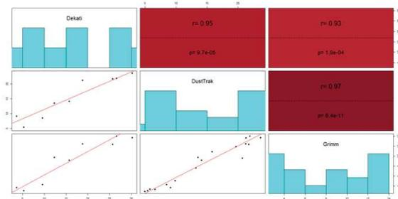
Figure 1: Correlation matrix for the comparison of values obtained by gravimetry (Dekati) with values obtained by optical methods (DustTrak and Grimm).
