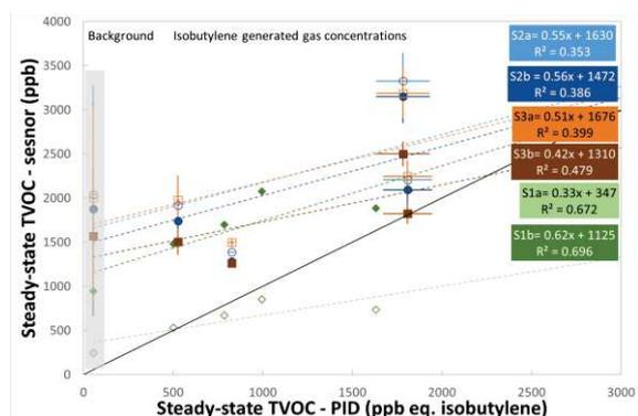
Figure 3. Steady-state TVOC sensor response to isobutylene reference gas. Sensors S4 and S6 were not equipped with TVOC detectors.
