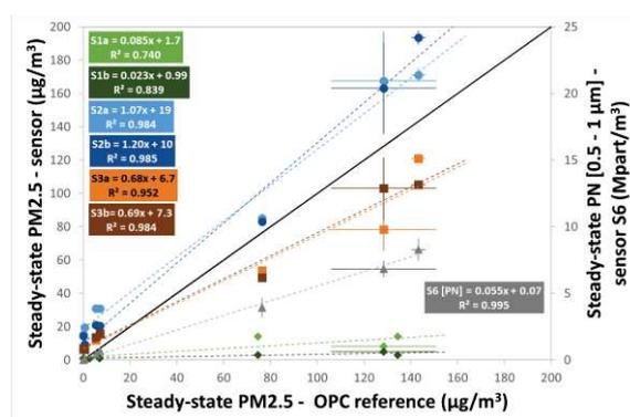
Figure 4. Steady-state sensor response to PM<sub>2.5</sub> generated from nebulization of salt solutions.
