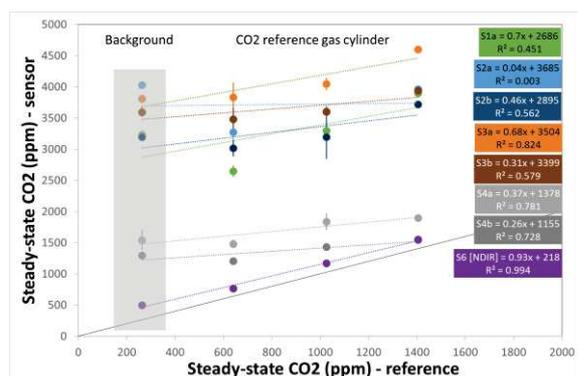
Figure 2. Steady-state sensor response to CO<sub>2</sub> reference gas.
