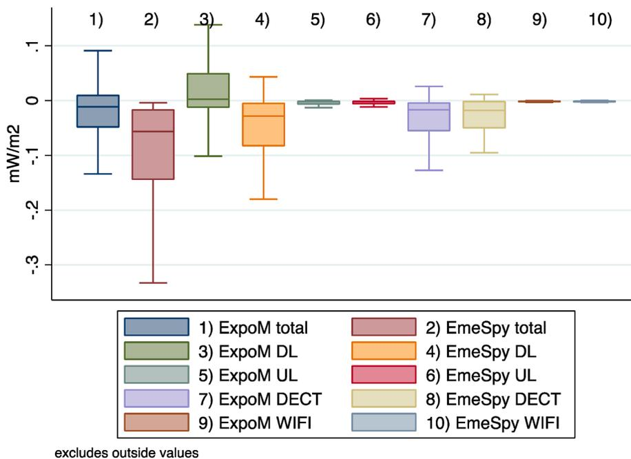
**Fig. 3.** Box plots of absolute differences of geometric mean levels per microenvironment, comparing exposimeter minus BWDM measurements for different exposure categories Total = total exposure, DL = Downlink, UL = Uplink, DECT = cordless landline phone. WiFi = WiFi 2.4G. For better visibility, outliers were removed.
