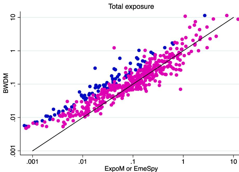
**Fig. 1.** Total ExpoM and EmeSpy exposure vs BWDM exposure Scatter plot of geometric means per microenvironment measured with ExpoM (magenta dots) or EmeSpy (blue dots) compared to measurements taken with the BWDM. The black line denotes  $y = x$ . Values are in  $mW/m^2$  and correspond to all frequency bands that are common to the three devices. (For interpretation of the references to colour in this figure legend, the reader is referred to the web version of this article.)
