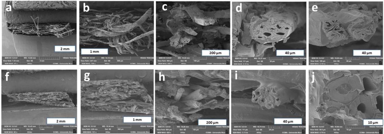
**Figure 2.** SEM images of surface of Jute/humins (top images a, b, c, d, e) and Jute/PFA composites (bottom images f, g, h, i, j) after fracture. The length of the white bar represents the scale indicated by each bar.
