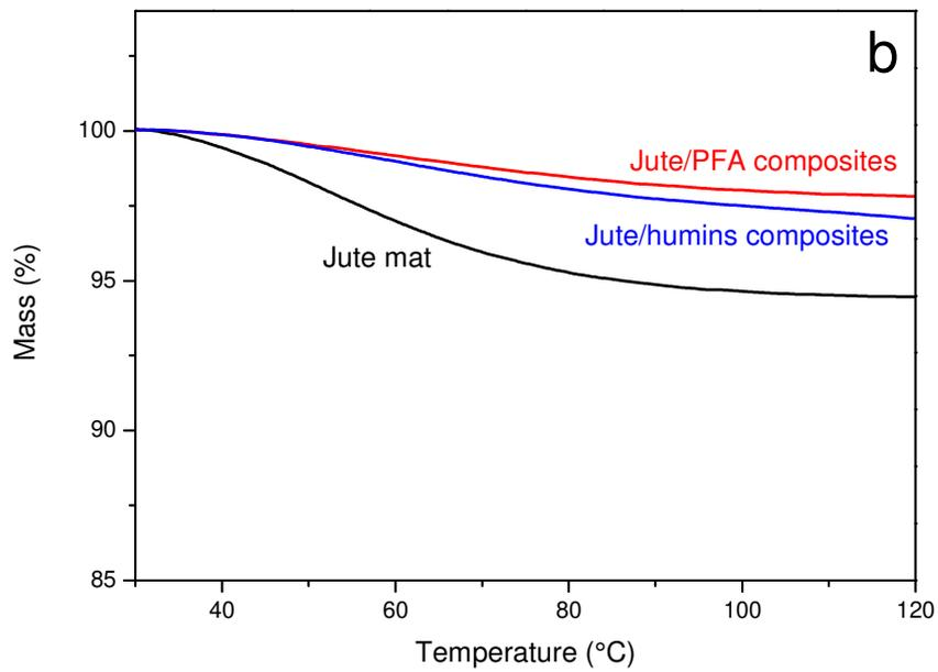
**Figure 3a.** TG and DTG curves of Jute/PFA and Jute/Humins composites. Neat Jute is given as reference. **3b.** Zoom of TG curves of Jute/PFA and Jute/Humins composites in the low temperature region. Neat Jute is given as reference.
