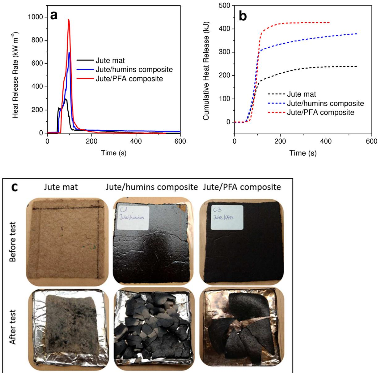
**Figure 5:** a) Heat Release rate (solid lines) and b) cumulative heat release (dash lines) profiles of jute mat, jute/humins composite and jute/PFA composite under fire conditions c) jute mat, jute/humins composite and jute/PFA composite before and after the FPA tests.
