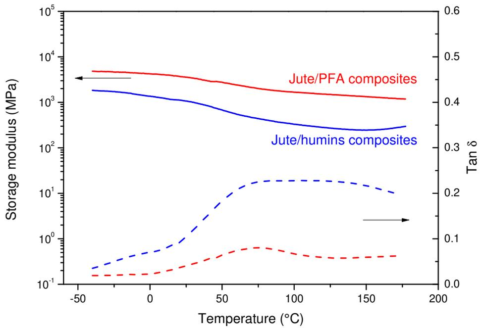
**Figure 1.** Evolution of storage modulus ( $E'$ ) and damping factor for Jute/PFA and Jute/Humins composites with temperature.
