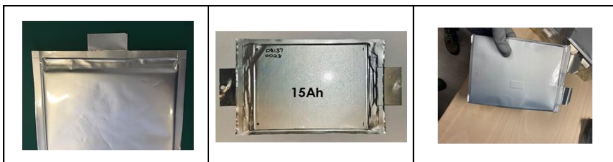
810 Figure 32: 3 generations of cells for DEMOBASE project with opposite (LS, LU and MU 811 types) tabs and “rabbit type” tabs configuration (Mter type).
