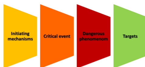
Figure 1. Simplified representation of an accident chain (Gombert et al, 2017)
