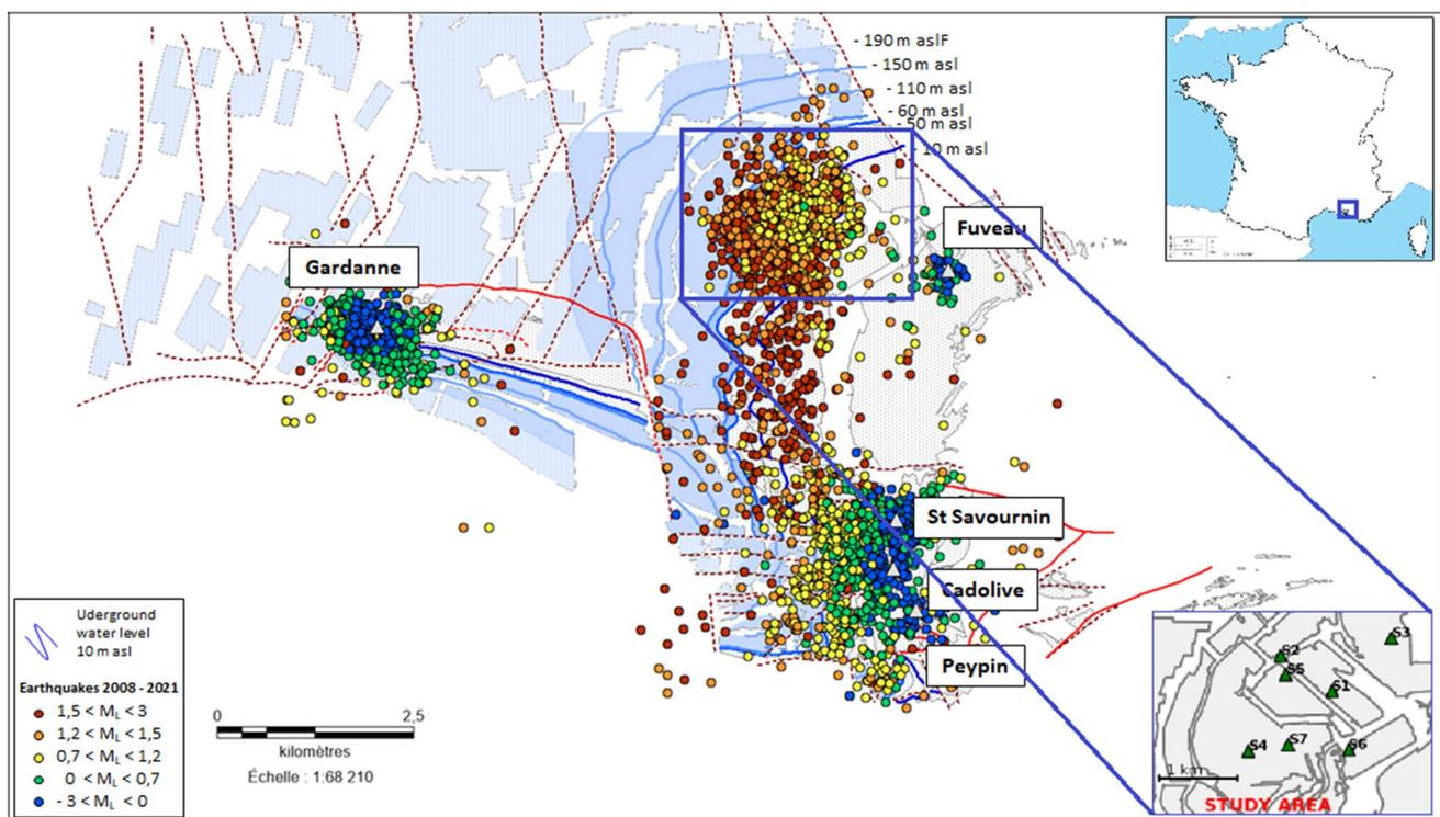
**Fig. 1** Flooded abandoned Gardanne mine with observed seismicity and monitoring networks. Stations of permanent monitoring network are marked with white triangles and the names are written next to it, accordingly. Temporary network installed in study area is shown within inset figure in lower right corner, where grey areas indicate excavated parts of mine. Flooded part of mine works shown in blue. Seismicity shown as a function of magnitude by colored dots,
