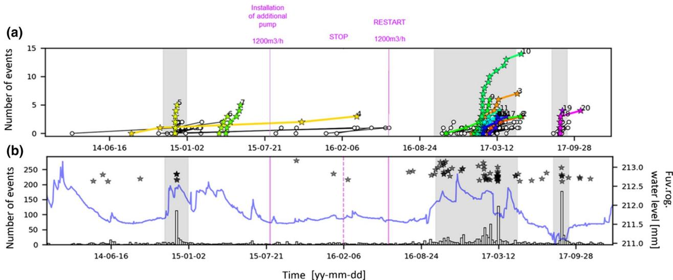
**Fig. 7** Temporal distribution of seismic activity **a** Events of each family and **b** Compared with water levels measured at Fuveau Rognacien well (around 2 km distance), corresponding to the rainfall data. Pumping capacity changes are marked with pink lines
