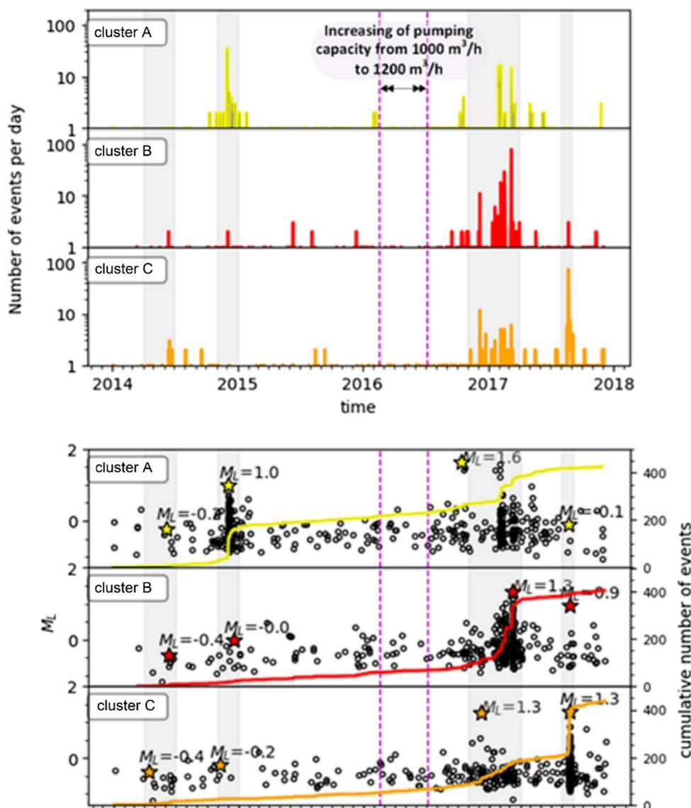
**Fig. 3** Temporal distribution of seismic activity for A and B class events, for central and north clusters: **a** Total seismic activity per day (top), and each cluster separately (figures below), compared with
